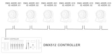
The figure above shows a simple DMX layout which has used three units at each DMX address. The three units have different ID addresses which allows the user to collectively control the whole group of units at that DMX address by setting CH10 to 0~4, or to control each unit independently by first selecting the DMX address and then by using CH10 to locate the target ID address
