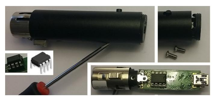
Note: The "DMX chip" is an 8 pin electronic integrated circuit (IC) component located on the electronic card, with the purpose of "driving" the DMX-512 signal.
