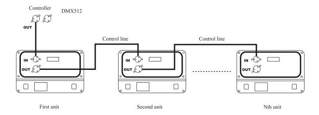
Caution: Please remember the signal output of last machine must connect the attached circle plug .The circle plug connect a 120 resistor between 2 feet and 3 feet canon plug. The signal reflects phenomena can be avoided by using circle plug during DMX 512 signal transfer. (DMX TERMIN ATOR CONNECTION):
