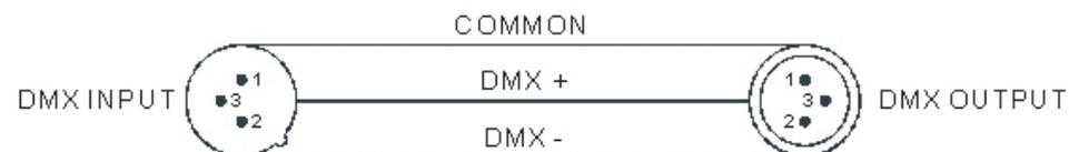
**Termination reduces signal errors and avoids signal transmission problems and interference. It is always advisable to connect a DMX terminal. (Resistance 120 ohm 1/4W) between pin2(DMX-) and Pin3(DMX+) of the last fixture.**
