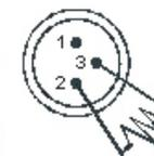
1. Connect the fixture together in a “daisy chain” by XLR plug cable from the output of the fixture to the input of the next fixture. The cable cannot be branched or split to a “Y” cable. Inadequate or damaged cables, soldered joints or corroded connectors can easily distort the signal and shut down the system
