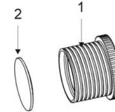
You should screw the lens roller to take it down as NO.1, and bring the lens out as No.2. Then you could replace the lens that you want to.
