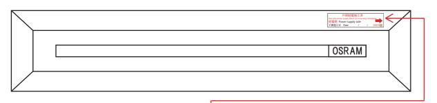
5. After the bypass work is completed, paste the sticker on the reflector of the lighting equioment. There is "OSRAM sticker" on power supply side of the LED lamp, so please make sure not to install the other side
