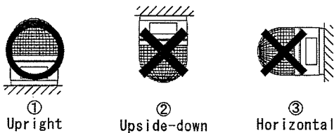
Mounting direction in outdoor (Please use a rubber mount)
