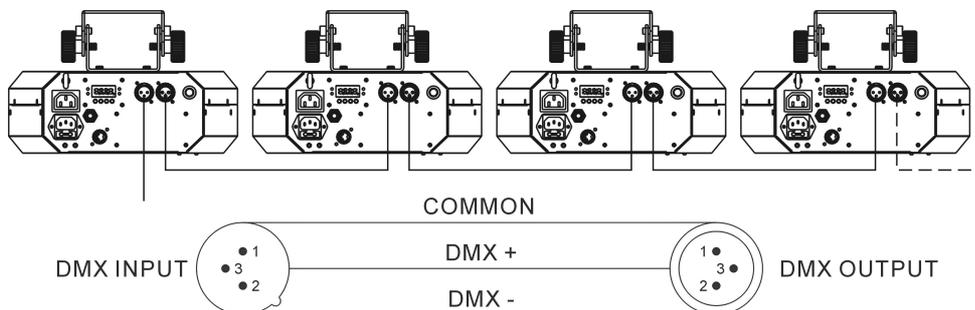
Termination reduces signal errors and to avoid signal transmission problems and interference. It is always advisable to connect a DMX terminal. (Resistance 120 ohm 1/4W) between pin2(DMX-)and pin3(DMX+) of the last fixture.
